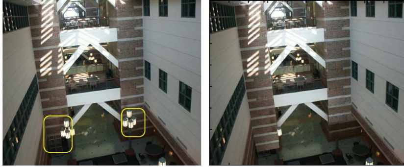
Fig. 4. Using multiple translation symmetry to remove the occlusion caused by lights.
