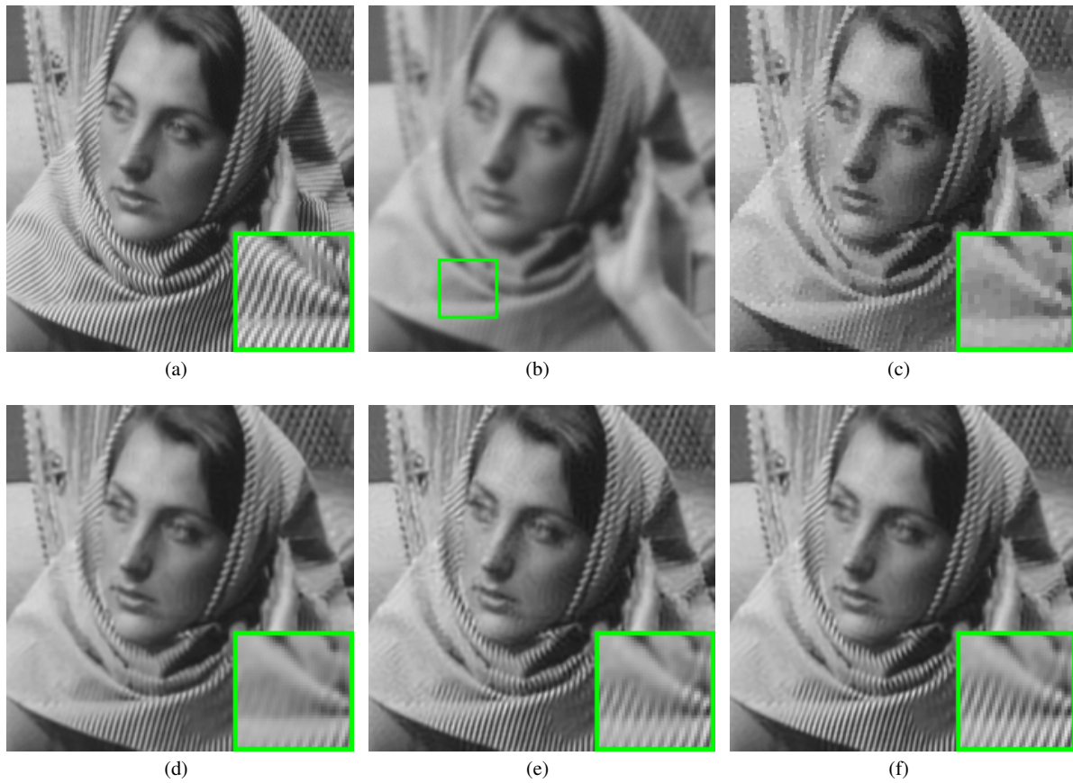
Fig. 5 Deblurring performance comparison on the Barbara image. (a) Original image; (b) Noisy and blurred image (Gaussian blur, \sigma_n = \sqrt{2} ); deblurred images by (c) FISTA [42] (PSNR=25.03 dB, SSIM=0.7377); (d) IDD-BM3D [33] (PSNR=27.19 dB, SSIM=0.8231); (e) NCSR [34] (PSNR=27.91 dB, SSIM=0.8304); (f) Proposed SSC-GSM (PSNR= 28.42 dB, SSIM= 0.8462 ).
