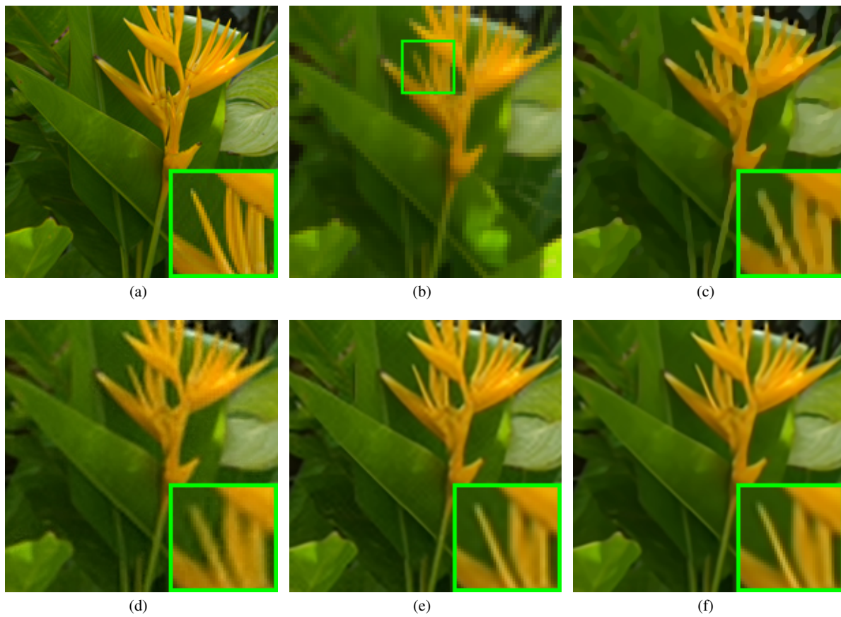
Fig. 6 Image super-resolution performance comparison on the Plant image (scaling factor 3, \sigma_n = 0 ). (a) Original image; (b) Low-resolution image; reconstructed images by (c) TV [43] (PSNR=31.34 dB, SSIM=0.8797); (d) Sparsity-based [44] (PSNR=31.55 dB, SSIM=0.8964); (e) NCSR [34] (PSNR=34.00 dB, SSIM= 0.9369 ); (f) Proposed SSC-GSM (PSNR= 34.33 dB, SSIM=0.9236).
