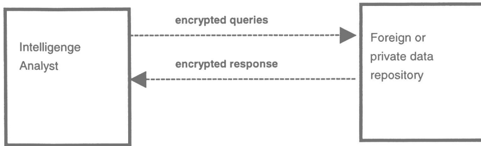
Fig. 1. A schematic representation of the Song/Perrig/Wagner secure query system
