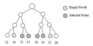
**Figure 3.** Providing completeness of query replies. Depicted is the result of a query *Select* \* where  $15 \le attribute \le 20$ . Empty proofs are returned for boundary nodes 14 and 21.
