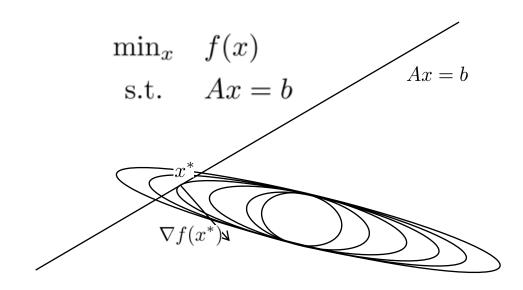
x\* with Ax\*=b is (local) optimum if and only if:  $\forall \Delta x$  if  $A\Delta x = 0$  then  $\nabla f(x^*)^{\top} \Delta x = 0$ .
