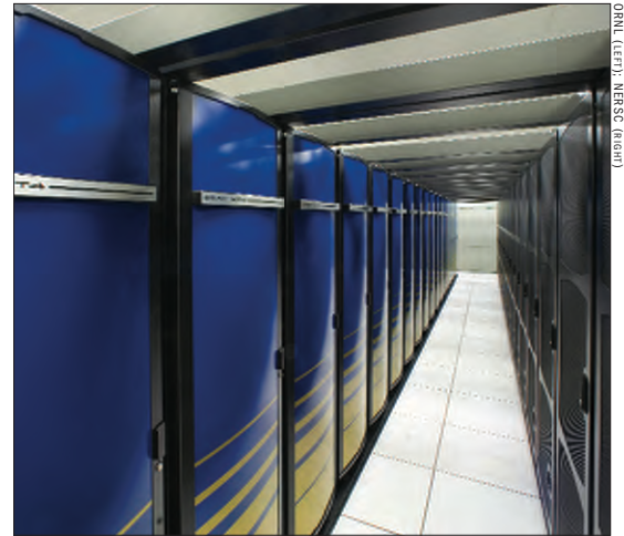
Figure 8. In the past year the Cray XT supercomputers at ORNL (Jaguar, left) and NERSC (Franklin, right) have both been upgraded from dual- to quad-core processors.
