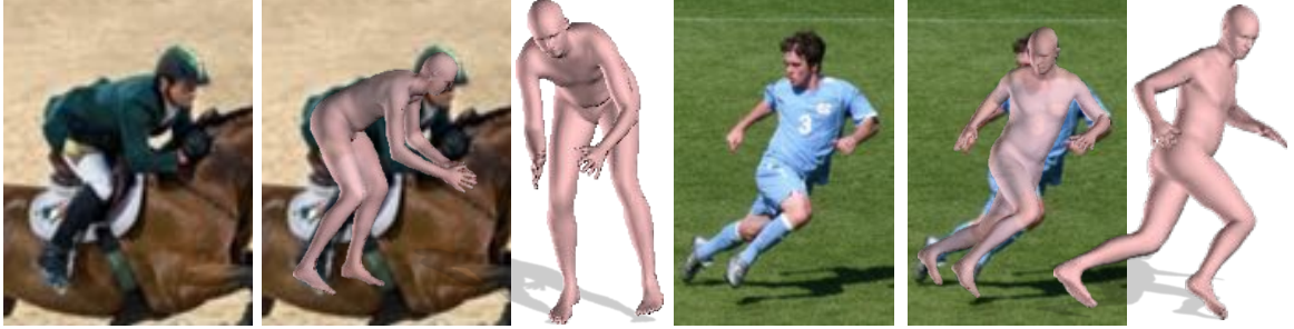
Figure 3-1: Example results. 3D pose and shape estimated by our method for two images from the Leeds Sports Pose Dataset [112]. We show the original image (left), our fitted model (middle), and the 3D model rendered from a different viewpoint (right).
