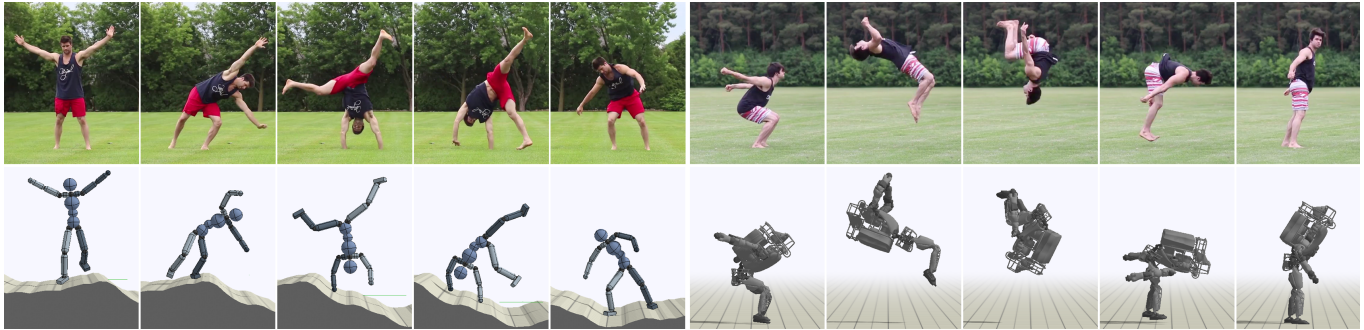
Fig. 1. Simulated characters performing highly dynamic skills learned by imitating video clips of human demonstrations. Left: Humanoid performing cartwheel B on irregular terrain. Right: Backflip A retargeted to a simulated Atlas robot.
