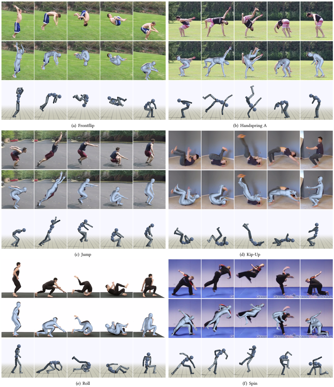
Fig. 6. Simulated characters performing skills learned from video clips. Top: Video clip. Middle: 3D pose estimator. Bottom: Simulated character.
