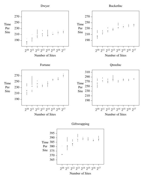
Figure 9: Comparison of the expected run times of different algorithms on sites chosen at random from a uniform distribution in the unit square. Times are in microseconds.
