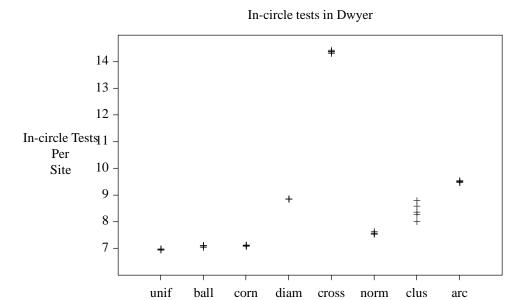
Figure 14: Dwyer in-circle tests on non-uniform inputs, n is 10K.
