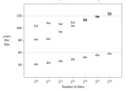
Figure 19: Run times for Dwyer (dw), BucketInc (inc), and Fortune using a heap (for) on a DEC Alpha for uniformly distributed sites.
