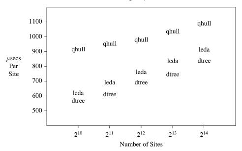
Figure 10: Comparison of the expected run times of Dtree, LEDA, and Qhull on sites chosen at random from a uniform distribution in the unit square.
