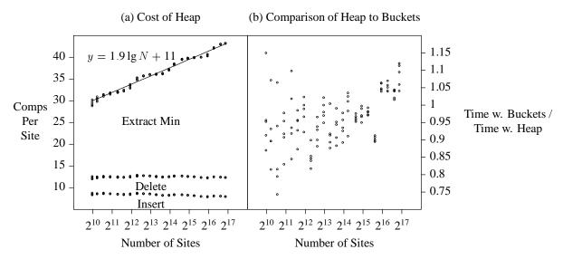
Figure 8: Cost of Fortune using a heap. Part (a) shows a breakdown of the cost of using a heap to represent the event queue. Part (b) plots the ratio of the run time of the old algorithm to the new.
