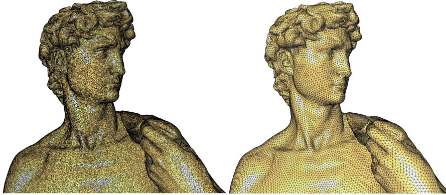
Fig. 1. Uniform remeshing of the Digital Michelangelo David model. Figure reproduced from [SAG03].
