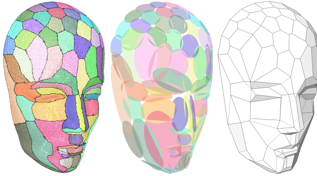
Fig. 18. Error-driven remeshing: Through repeated error-driven partitioning (left), a set of geometric proxies (represented as ellipses, center) is optimized. These proxies are then used to construct an approximating polygonal mesh (right). Figure reproduced from [CSAD04].
