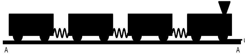
Figure 3.6: “Train”: 4 masses (3 “cars” and “engine”) linked by elastic springs and sliding without friction (aside of controlled force u ) along “rail” AA.
