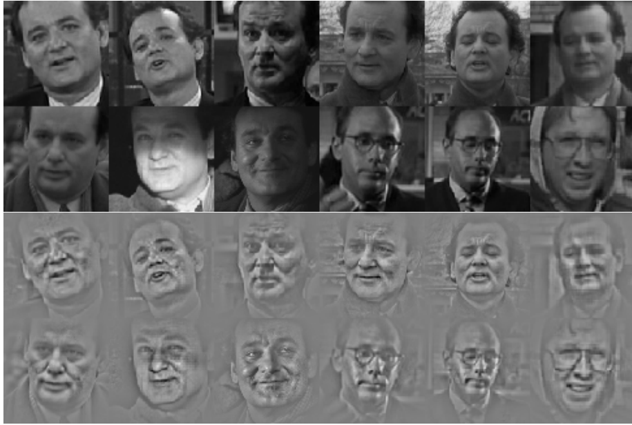
Fig. 5. Pre-processing. Upper set: original (raw) extracted faces. Lower set: faces after bandpass filtering and feathering. Variations in lighting across the image are removed, and boundary effects are diminished.
