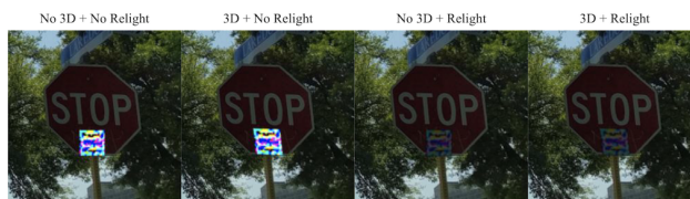
Figure 4: Example ablation of the geometric and relighting transforms in our dataset. The rightmost stop sign has a patch rendered with a perspective and relighting transform which makes it more realistic. The first and second images have patches that are too bright whereas the first and third images have patches that do not respect the sign’s orientation.
