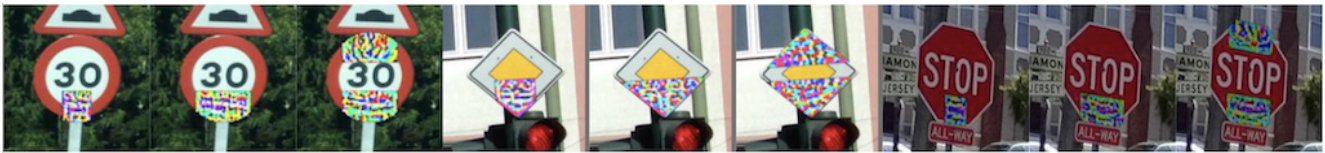
Figure 7: Examples of small (10'' \times 10''), medium (10'' \times 20'') and large (two 10'' \times 20'') patches applied to three of the signs from our benchmark. The large patch size is clearly visible and obscures the notion of imperceptibility. We still choose to experiment with it since it is approximately the same size used by prior work [17, 66].
