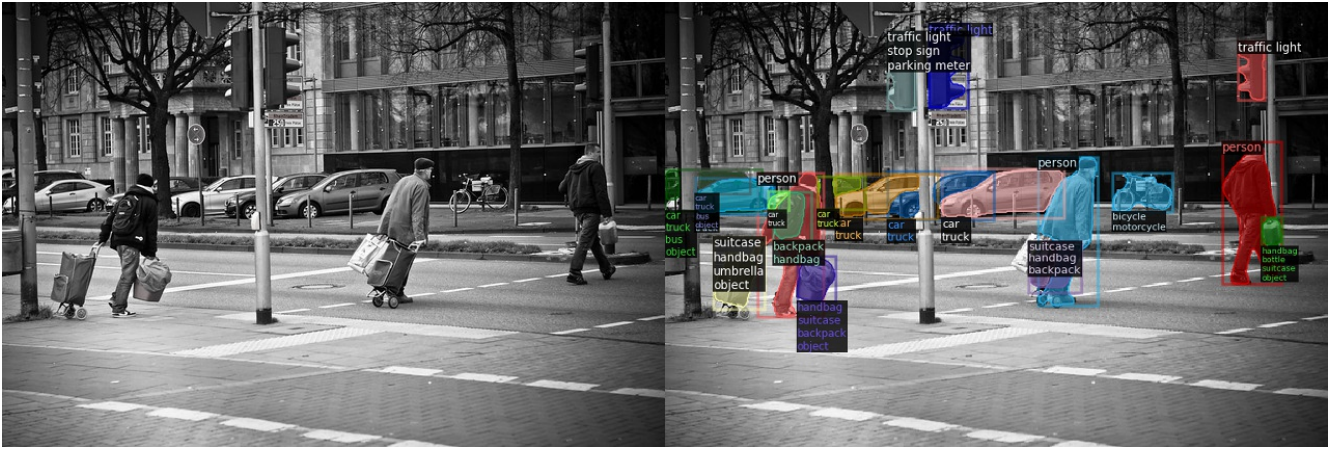
Figure 1: Object detection with simultaneous distribution-free guarantees on the expected intersection-over-union, recall, and coverage rate is possible with our methods; see Section 7 for details.
