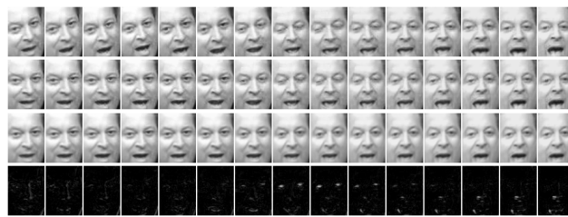
Figure 5. Stabilization of faces in the video. 1st row: frames 1-15 from a 140-frame video, aligned by applying a face detector to each frame; 2nd row: RASL alignment result D \circ \tau ; 3rd row: recovered images A of rank 64; 4th row: sparse error E .
