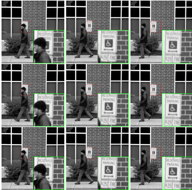
Figure 8. Recovery of the 12-frame building video acquired by a handheld camera using our 3DSM at M/L = 30\% . Top: initial results without image alignment (a) (PSNR: 31.50 dB), (b) (PSNR: 31.71 dB) and (c) (PSNR: 32.63 dB). From initial results, the estimated translations (\Delta x, \Delta y) are listed as (a)(2.35, 3.11), (b) (0.62, -1.77), (c)(-0.31, 2.36). Middle: final results with estimated (\Delta x, \Delta y) (a) (PSNR: 33.85 dB), (b) (PSNR: 34.10 dB) and (c) (PSNR: 35.18 dB). Bottom: three original frames.
