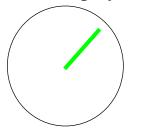
Streak had length proportional to intercepted signal's strength, and pointed to its direction, and persisted slightly longer.
