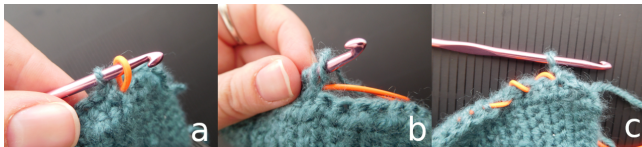
Figure 4: Different techniques to integrate a flexible LED. Using material instead of/combined with yarn in a crochet stitch (a), laying material on the previous crochet row and crocheting around it (b), wrapping material around crochet stitches (c).
