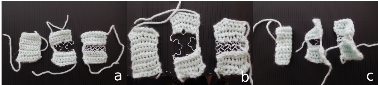
Figure 6: Crochet and crochet with infill patterns Cross and Gyroid behave differently, a) lying flat, b) stretched and c) bent.
