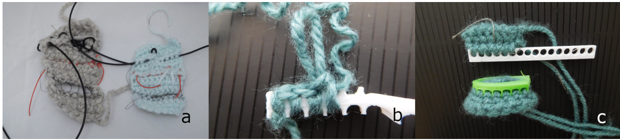
Figure 5: Materials as part of or to replace crochet: Integrating material into crochet, top to bottom: cTPU (black, thick), insulated cable (red), thread (black thin) (a). 3D-printed parts can replace a row of crochet stitches, even without closed holes (b). Stiff PLA or flexible TPU can guide the work in different ways (c).
