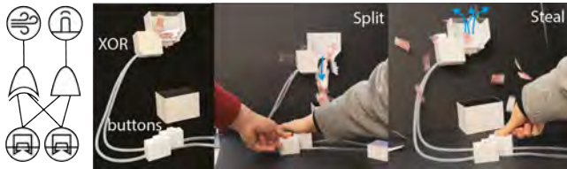
Figure 11: The Split or Steal game drops money if both players choose split (AND), or blows the air in and spreads the money if a player chooses steal. (XOR).
