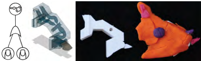
Figure 12: This clay dog head is modeled over a bare set of widgets that detect touch A OR touch B and actuate an oscillator; the same widgets form the core of the bunny.
