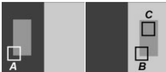
Figure 1. Correspondence is difficult when a uniform surface moves across different background patterns. Consider the correspondence of window A with windows B or C; traditional robust methods equate the match between A:B and A:C, since the “outlier” regions in each is equally different.
