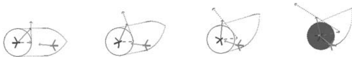
Fig. 8. Pursuer starts within the reachable set, and thus can cause a collision despite the best efforts of the evader (animation at [44]).
