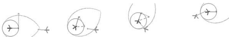
Fig. 14. Evader keeps pursuer from entering the projective overapproximation \mathcal{Y}_{12} of the reachable set, and hence conservatively avoids collision.
