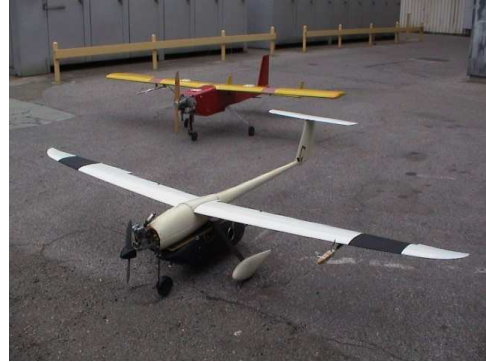
Fig. 1. A photograph of the Stanford DragonFly UAVs (DF2 and DF3). The aircraft are approximately 10 foot in wingspan, with onboard navigation, communication, and control algorithms, all designed by us.
