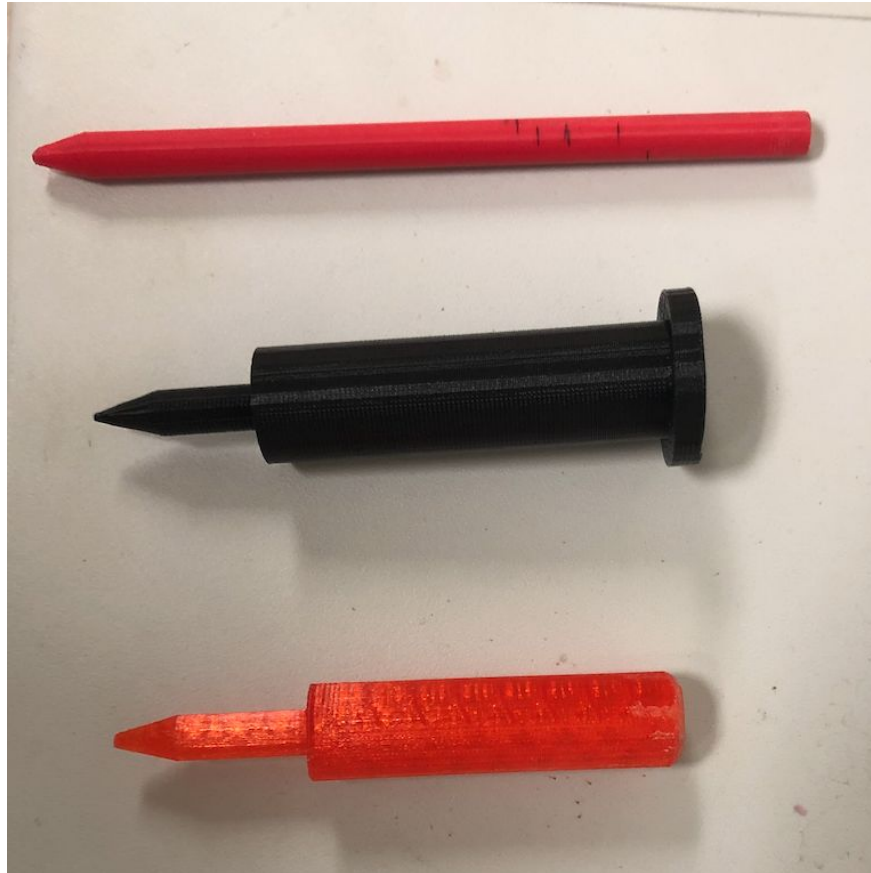
Fig. 31. Multiple iterations of the sensor probe for the testing box
