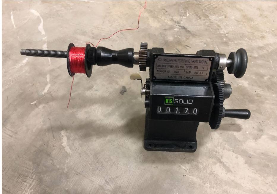
Fig. 40. Mechanism obtained for easier and more standardized coiling of the wire.
