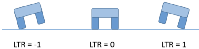
Figure 1: LTR represents the load distribution between wheels. 0 corresponds to load being equally distributed and \pm 1 corresponds to load being completely on one set of wheels.
