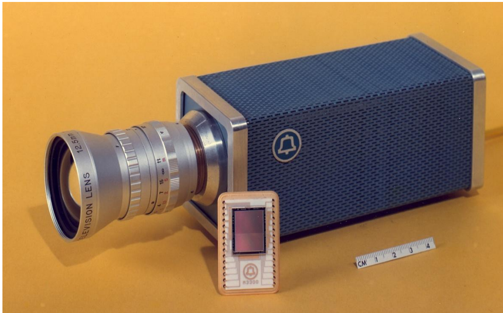
Figure 1: The first solid state image sensor compatible with the American broadcast TV format.
