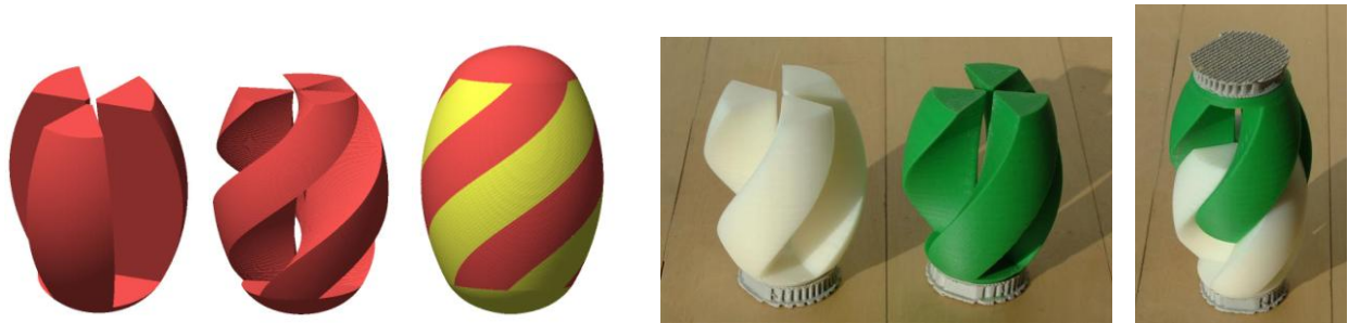
Figure 7: Multi-prong helicoidal dissections: CAD models: (a) linear slide-apart geometry; (b) one part twisted; (c) two parts intertwined. Realization of this concept: (d) the two pieces shown individually; (e) the two pieces partly intertwined.
