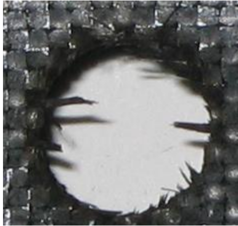
Figure 3.11: Defect during low-feed drilling
