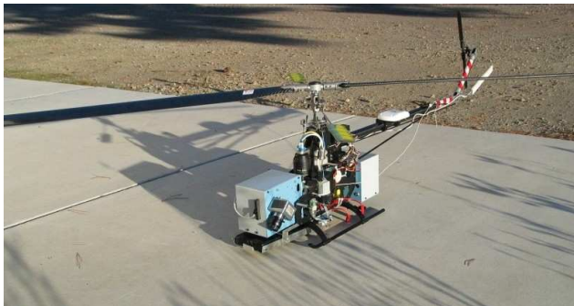
Figure 1: An electrically-powered, MPC-controlled UAV testbed for vision-based landing and terrain mapping.
