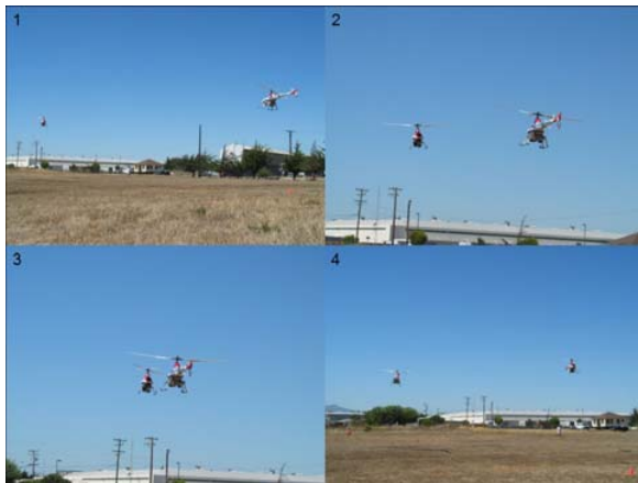
Fig. 8. Mid-air collision avoidance between two rotorcraft UAVs using real-time MPC
