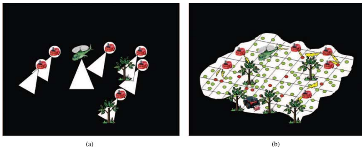
Fig. 1. (a) Sensor visibility in PEGs without sensor network. (b) Sensor visibility in PEGs with sensor network. Dots correspond to sensor nodes, each provided with a vehicle detection sensor. Courtesy of [20].
