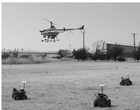
Fig. 1. A Berkeley RUAV in an autonomous mission with Unmanned Ground Vehicles
