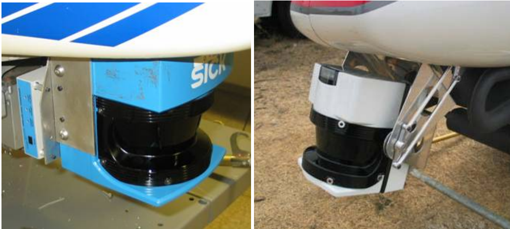
Figure 3. Laser scanning devices mounted on Berkeley UAVs (left: fixed, right: actuated mounting)
