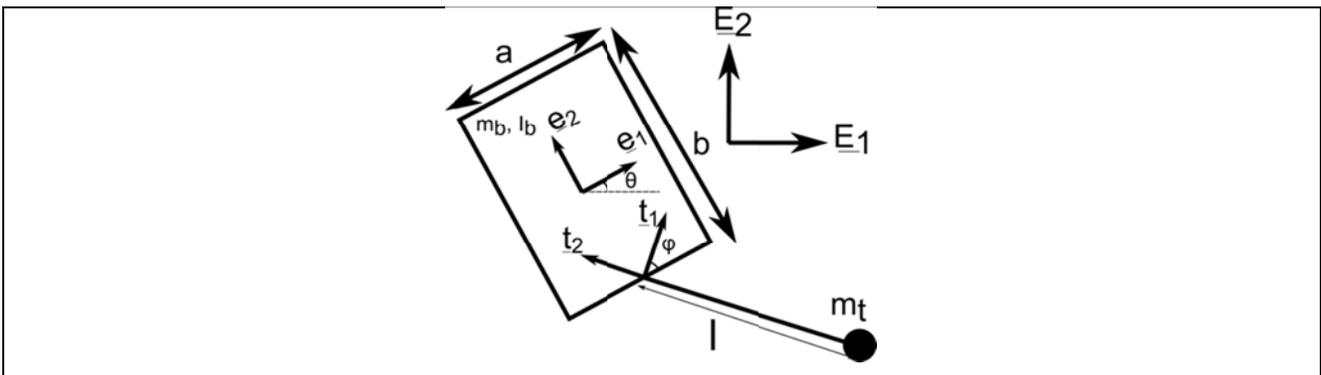
Fig. 8: Model of the robot with tail.  $I_b$  and  $m_b$  are the robot body's yaw inertia and body mass respectively.  $\theta$  is its body angle.  $m_t$  is the mass of the tail,  $l$  is the length, and  $\varphi$  is the angle of rotation of the tail with respect to the ground.
