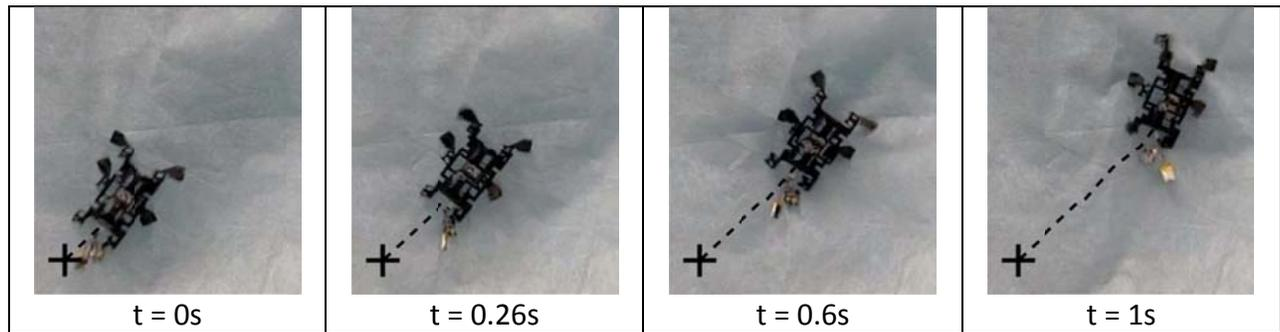
Figure 4 – A sequence of frames showing CLASH climbing loose vertical cloth.
