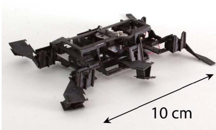
Figure 1 – CLASH with onboard battery mounted internally. The electronics are removed to reveal the body and transmission.
