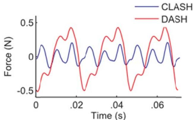
Figure 2 – The normal forces generated by DASH during operation (red) are significantly greater than those generated by CLASH (blue).
