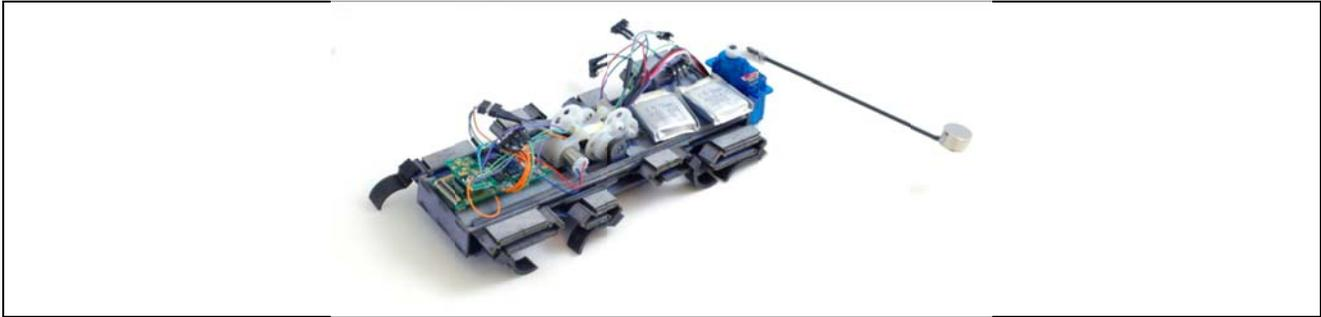
Fig. 7: The OctoRoACH equipped with a dynamic tail, allowing quick momentum exchange and turning capabilities on low-friction surfaces.
