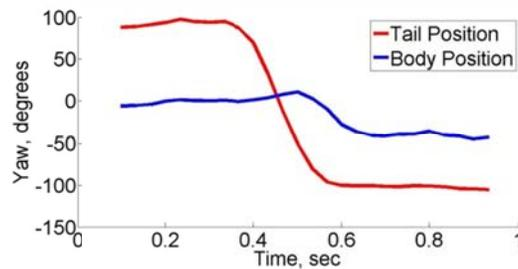
Fig. 10: A plot of tail and body position from the experiment in figure 2. Note that the robot begins to turn slightly when the tail is actuated, but most of the turning occurs after the tail decelerates.
