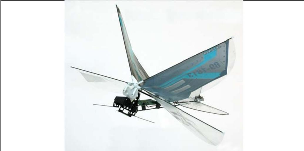
Fig. 5 BOLT: A bipedal ornithopter capable of both aerial and terrestrial locomotion.
