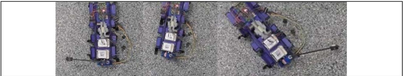
Fig. 9: The robot begins moving its tail CCW, inducing a small CW movement in the body. After impact, however, the body moves CCW significantly.
