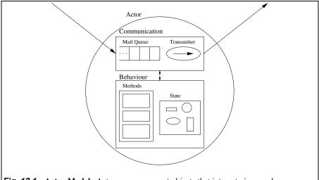
**Fig. 13.1** Actor Model: Actors are concurrent objects that interact via asynchronous messages.
