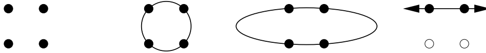
Figure 4: The search spaces for four optimization problems (ignoring the balance constraint). From left to right: The domain of the discrete optimization problem is the vertices of a hypercube. The domain of the relaxed optimization problem solved by the simplest spectral partitioner is a hypersphere passing through those vertices. The domain of the relaxed problem solved by a spectral partitioner with vertex masses is an ellipsoid. The domain of the relaxed problem solved by an isoperimetric partitioner is a hyperplane.
