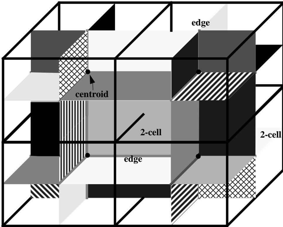
Figure 2. A four hex mesh and its dual. The 2-cells divide the volume inside the mesh into 3-cells, one for each hex node.
