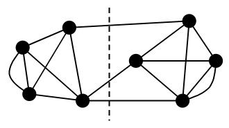
The minimum cut is shown by a dotted line. The cut itself is the set of edges that the dotted line crosses. Note that the graph above is actually a multi-graph, that is, there is more than one edge between some pairs of vertices. But there are no edges whose endpoints are the same vertex (no self-loops).
