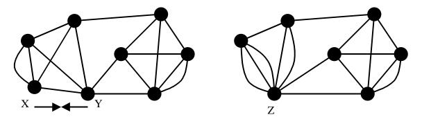
Notice that new multiple edges can result if both x and y are connected to the same vertex before the contraction. That is fine. The graph is a multigraph anyway, and we just keep all the edges that result.
