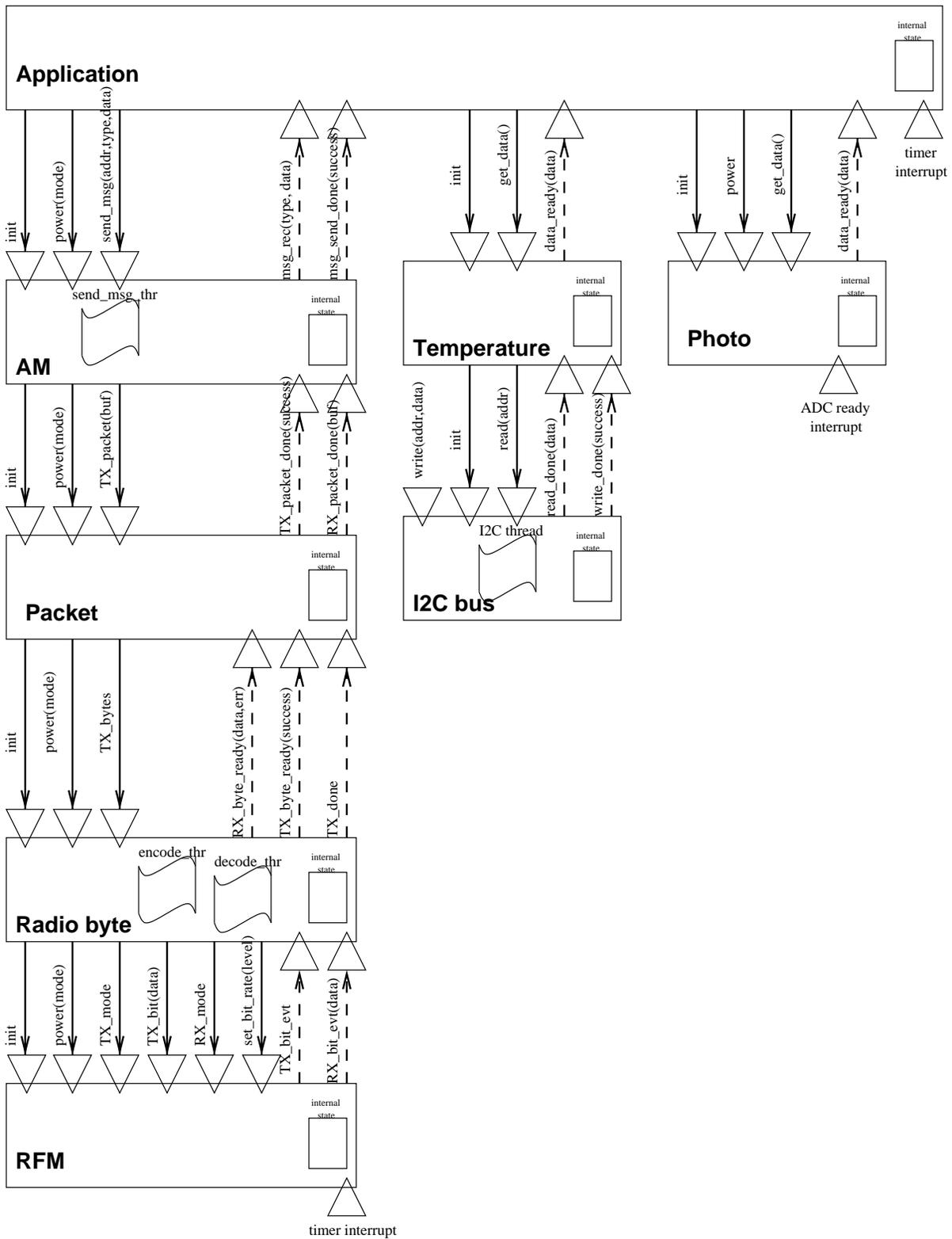
Figure 3: A sample configuration of a networked sensor
