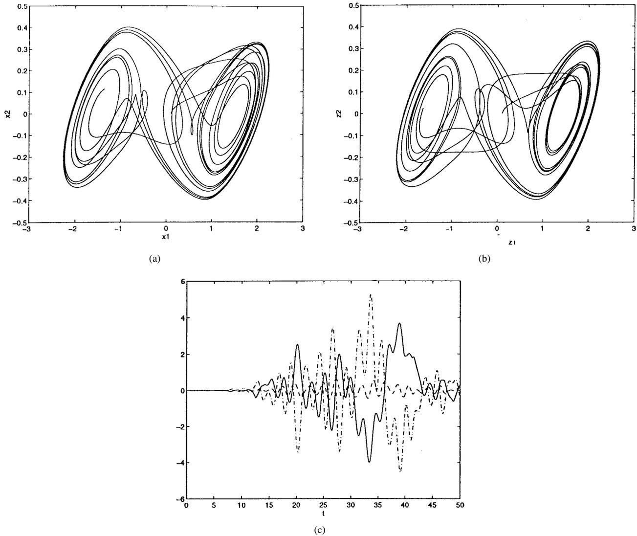
Fig. 4. Static state error feedback (continued). Behavior of the master and slave systems in the autonomous case, for the parameter mismatch of Fig. 2(a) and initial condition  $x(0) = z(0) = [0.1; 0; 0]$ . (a)  $(x_1, x_2)$  of the master system. (b)  $(z_1, z_2)$  of the slave system. (c)  $x - z$  with respect to time.
