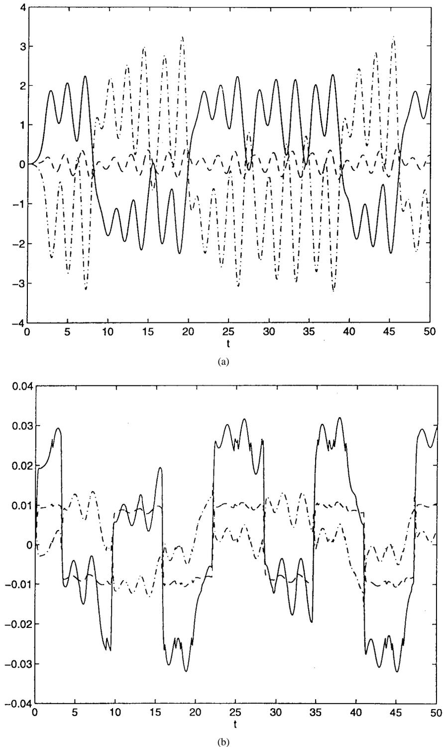
Fig. 3. Static state error feedback (continued). (a) Transmitted signals  $p$  which are a linear transformation of the state variables  $x$  of the master system, with  $p_1$  (-),  $p_2$  (- -),  $p_3$  (-.). Applying vector field modulation, the message signal is invisible on the chaotic carrier signal. (b) Control signal  $u$  applied to the slave system using full static state error feedback, with  $u_1$  (-),  $u_2$  (- -),  $u_3$  (-.).
