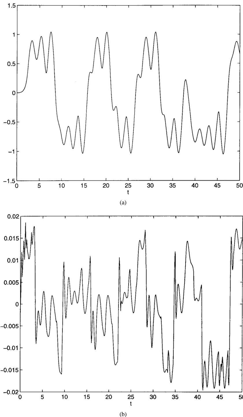
Fig. 7. Dynamic output feedback (continued). (a) Transmitted signal  $p$  which is a linear combination of the state variables  $x_1, x_2$  of the master system. Applying vector field modulation, the message signal is invisible on the chaotic carrier signal. (b) Control signal  $u$  applied to the slave system.
