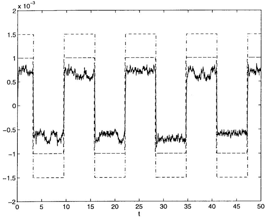
Fig. 5. Static state error feedback (continued). Simulation of the synchronization scheme for the same case as Fig. 2(a) but with zero mean white Gaussian channel noise  $\epsilon$  with standard deviation 0.0001.
