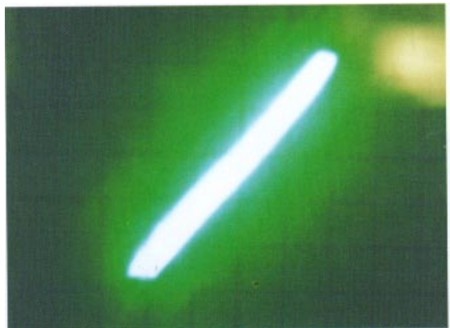
Fig. 5. The experimental results of impulsive synchronization when v_1 is sampled as the synchronizing impulse sequence. In this figure, the scale of the oscilloscope is 50 mV/div for both horizontal and vertical axes. (a) The driving system and the driven system are originally desynchronized. (b) Impulsive synchronization. (c) Impulsive synchronization with narrow impulses. (d) The switching signal s(t) used in (c).
