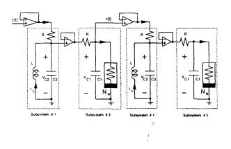
Figure 1: Electronic circuit implementation of the twostage "receiver" consisting of two identical copies of the circuit given in Fig. 2 (b) of [1].
