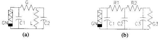
Fig. 5. (a) Chua's 3-D circuit; (b) associated RC-ladder obtained by transforming Chua's circuit.
