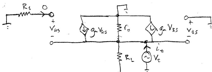
$$i_t + g_m V_{as} + g_{mb} V_{BS} - V_t \left( \frac{1}{r_0} + \frac{1}{R_L} \right) = 0$$
