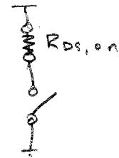
$$R_{DS(on)} = \frac{1}{\mu_n C_{ox} \frac{W}{L} (V_{DD} - V_{TH})}$$
