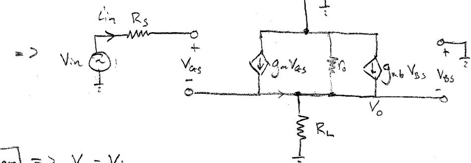
$$I_{in} = 0 \Rightarrow R_{in} = \infty \Rightarrow V_g = V_{in}$$
