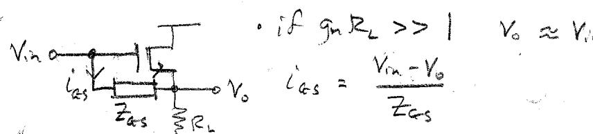
$$\text{if } g_m R_L \gg 1 \quad V_o \approx V_{in}$$
