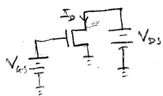
$$\text{Pinch off requirement: } V_{GD} < V_{TH} \Rightarrow V_{DS} \geq V_{GS} - V_{TH}$$
