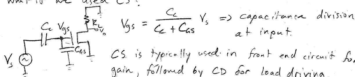
CS is typically used in front end circuit for gain, followed by CD for load driving.
