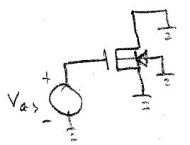
$$R_{DS} = \frac{1}{\mu_n C_{ox} \frac{W}{L} (V_{GS} - V_{TH})}$$
