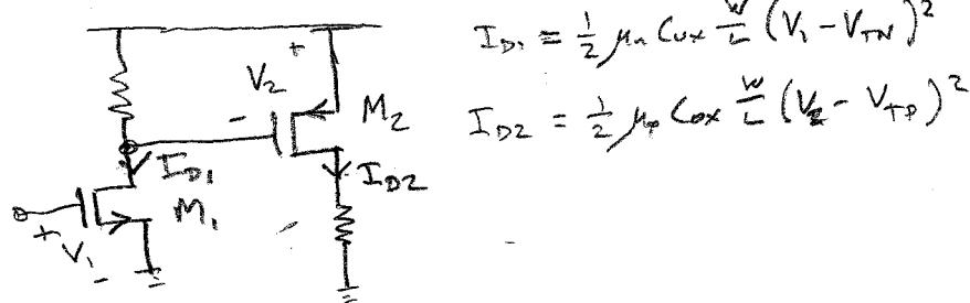
$$I_{D1} = \frac{1}{2} \mu_n C_{ox} \frac{W}{L} (V_1 - V_{TN})^2$$
