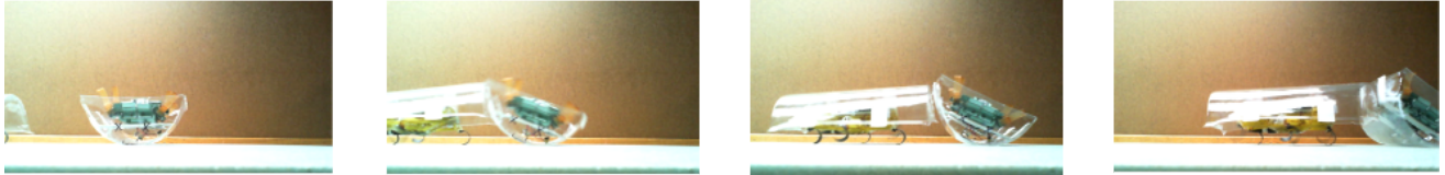
Fig. 10: Frame sequence of RoACH team failing to perform cooperative righting maneuver on styrofoam substrate due to insufficient ground-shell friction .
