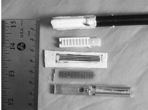
Figure 9: A tactile sensor mounted on a laparoscopic instrument, and components including (top to bottom) molded dielectric, upper copper layer, circuit board, and mount.
