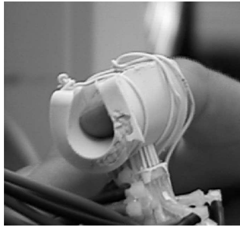
Figure 13: The tactile display attached to the finger.
