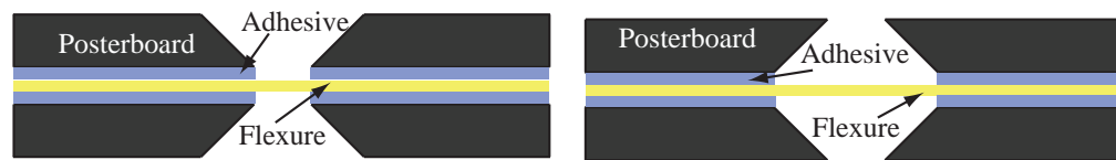
(a) A flexure in which the initial cuts were performed with inner adhesive faces down. (b) A flexure in which the initial cuts were performed with the inner adhesive faces up.
