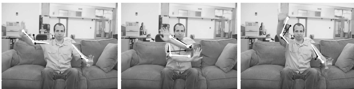
Fig. 8. (top) Twelve frames were annotated with the joint positions of the subject in a 1500 frame video sequence. (middle) The recovered positions of the hands and elbows for the unlabeled frames are plotted in white. The output of fully-supervised nonlinear regression using only the 12 labeled frames and no unlabeled frames is plotted in black. Using unlabeled data improves tracking significantly. (bottom) Recovered joint positions for frames that were not in the training set. The resulting mapping generalizes to as-yet unseen images.
