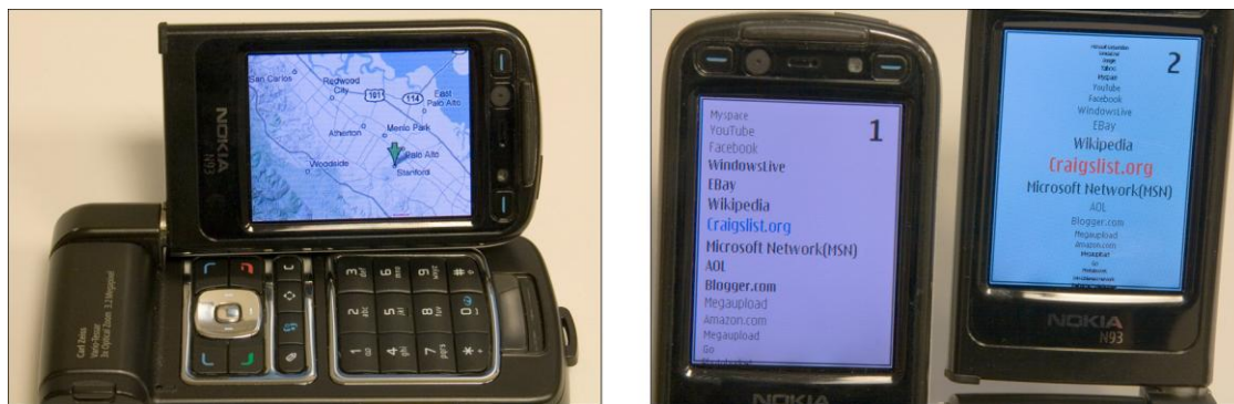
Figure 5.9: Two prototypes built with Juxtapose mobile. Left: A map navigation application explored use of variable tuning. Right: Two alternatives of a fisheye menu navigation technique running on two separate phones.
