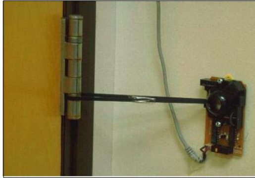
Figure 3.4: Buxton’s Doormouse [56] is an example of a “hardware hack” that repurposes a standard mouse.
